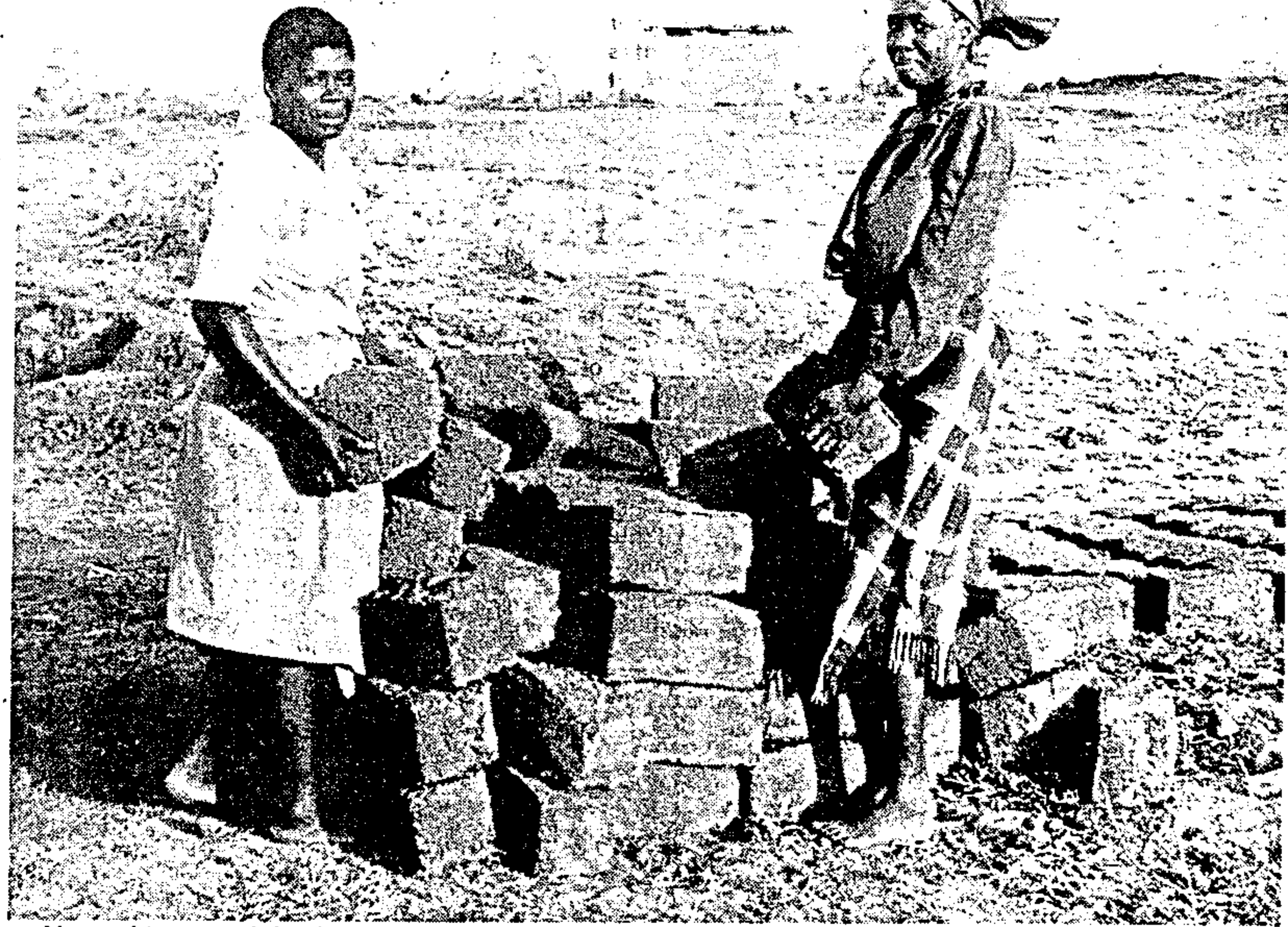
Mozambicans with bricks made of mud, stone and grass, which they use to build homes at Rhalani.
