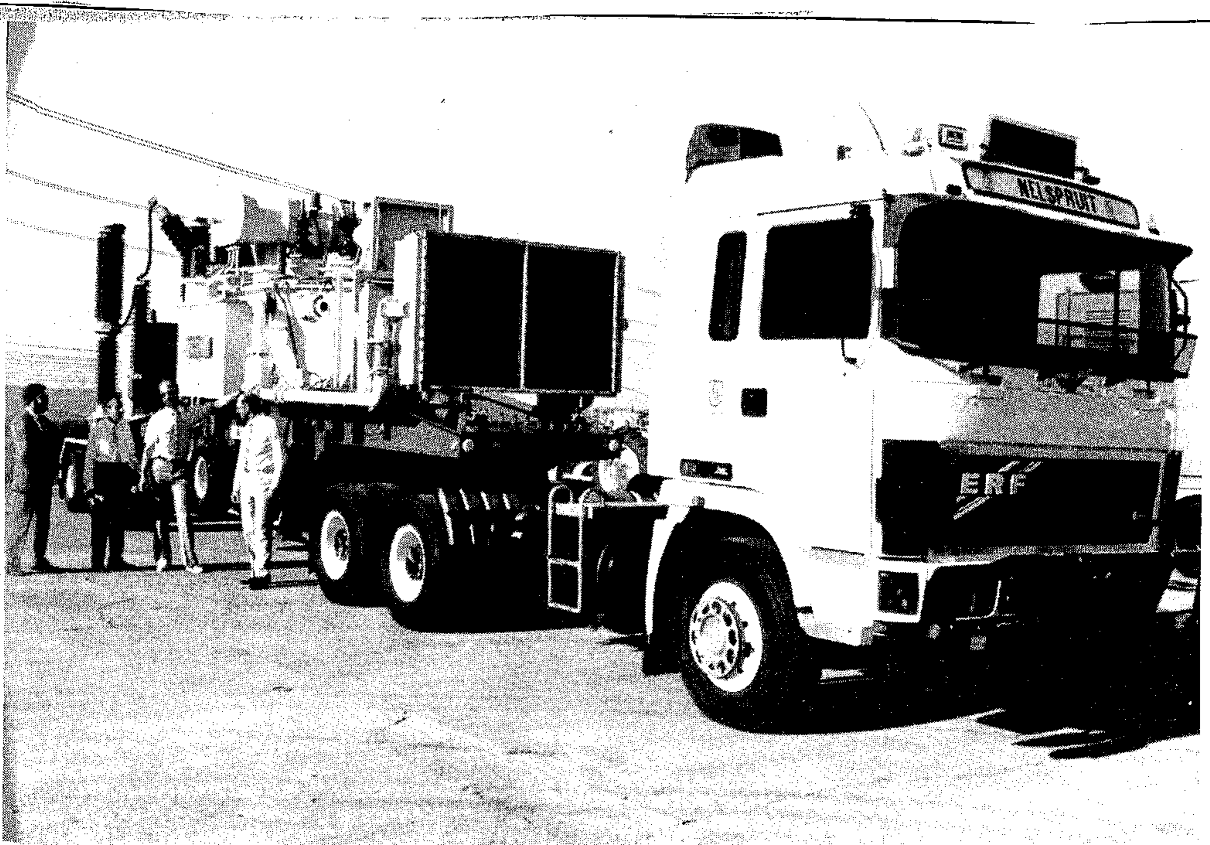
Eskom's 16,5 ton mobile generator capable of illuminating a town the size of Komatipoort.
