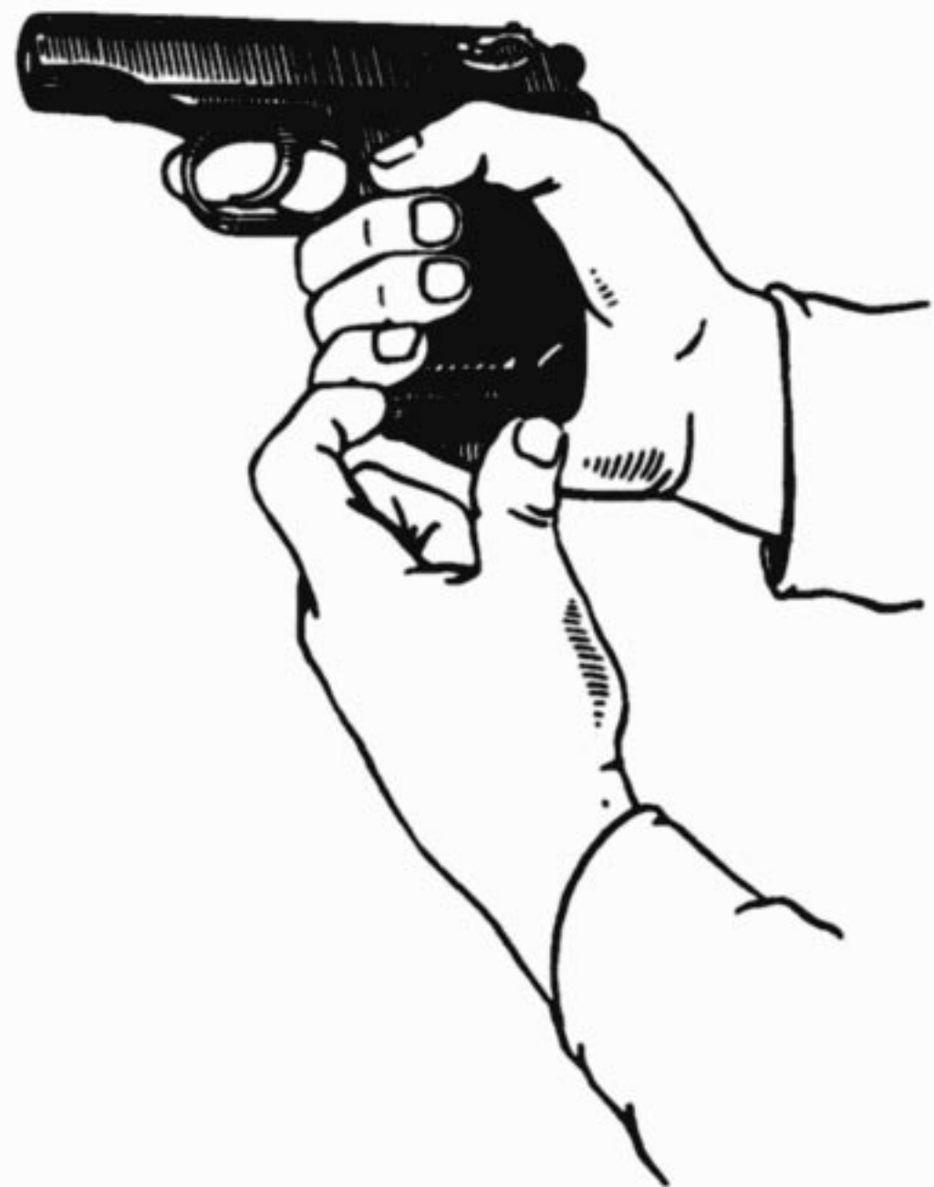
Fig. 3. Removing magazine from grip
