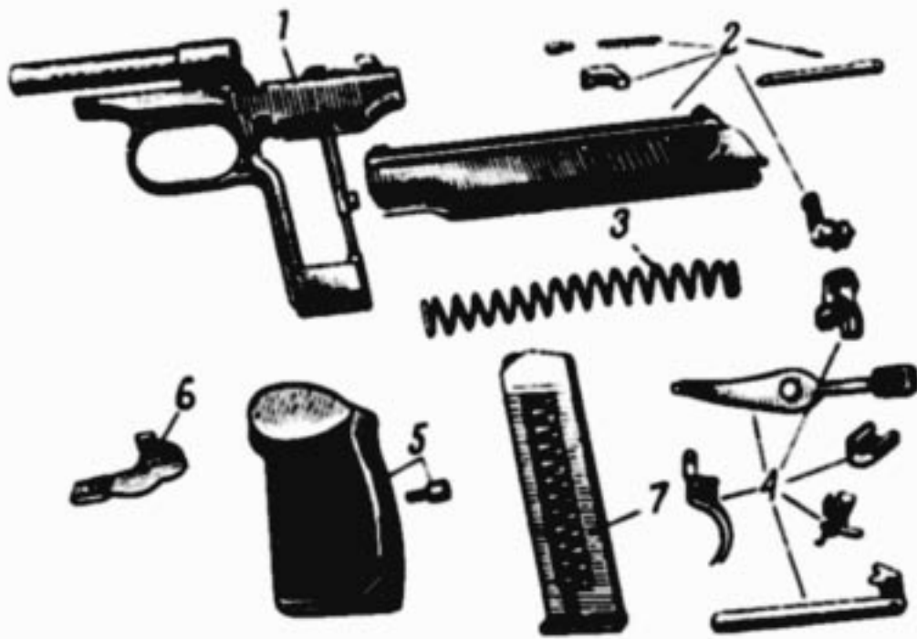
Fig. 2. Main parts and mechanisms. 1 - receiver, barrel and trigger guard assembly, 2 - slide, firing pin, extractor and safety lock, 3 - recoil spring, 4 - firing mechanism component parts, 5 - grip stocks and retaining screw, 6 - slide stop, 7 - magazine
