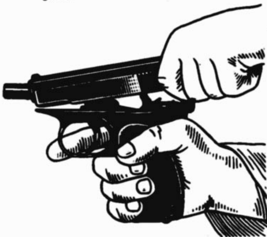
Fig. 5. Detaching slide from receiver
