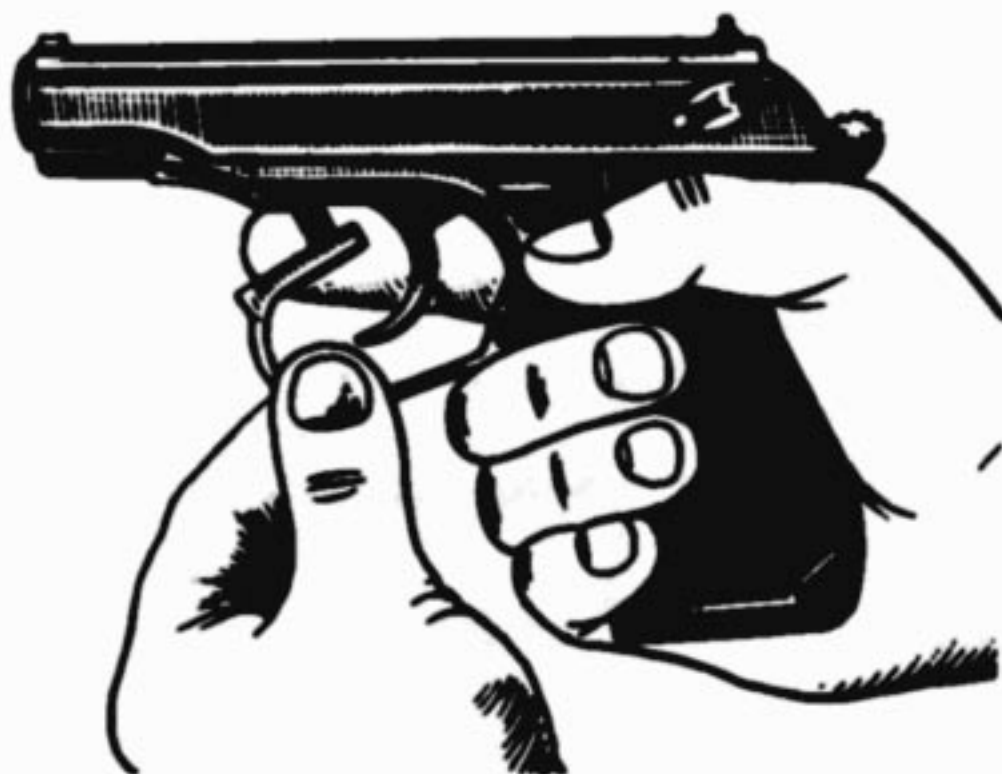
Fig. 4. Pulling down forward end of trigger guard
