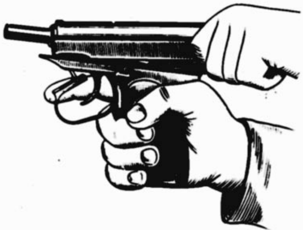
Fig. 6. Coupling slide to receiver
