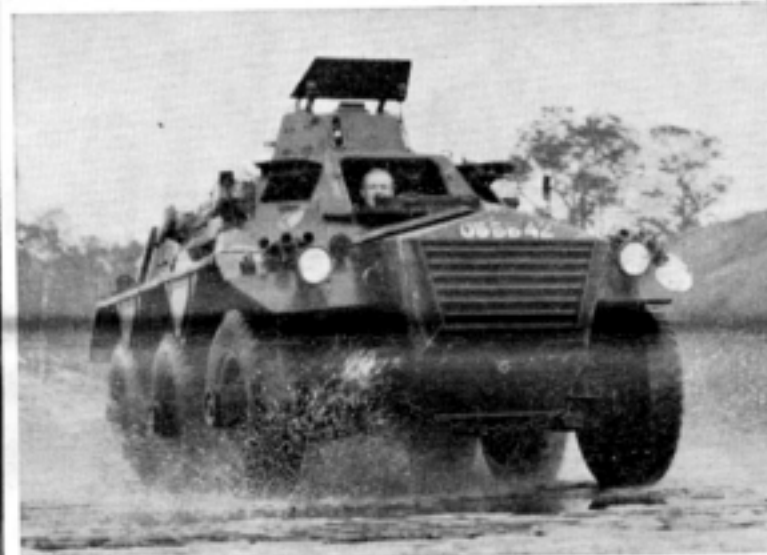
Saracen armoured cars have been supplied to the police and already used in riot-areas. They played a big part in the recent Paarl riots. Here is one travelling at speed — their top speed is 40 m.p.h.
