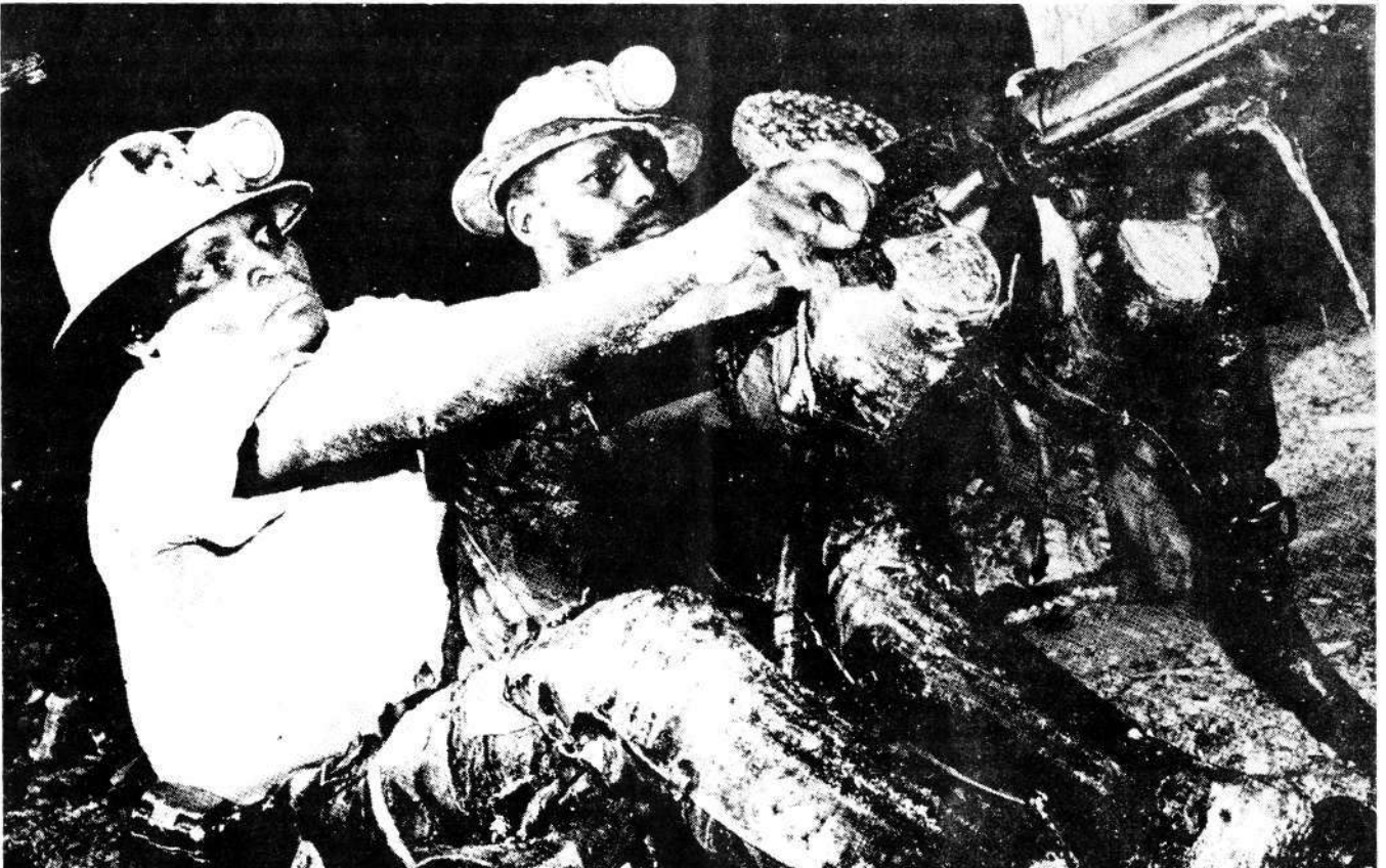
Drilling at stope face
