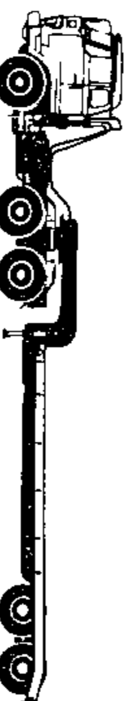
ZM 702 742 GVM 22 400 kg 201 kW engine Max body length 7.6 m
