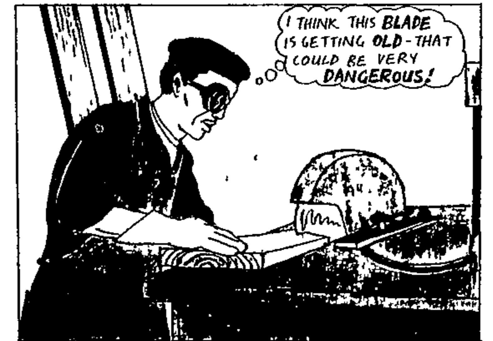
WORKERS SHOULD ALWAYS HAVE EYE PROTECTION WHERE THERE IS DUST OR FLYING CHIPS ALL SAWS MUST HAVE GUARDS.
